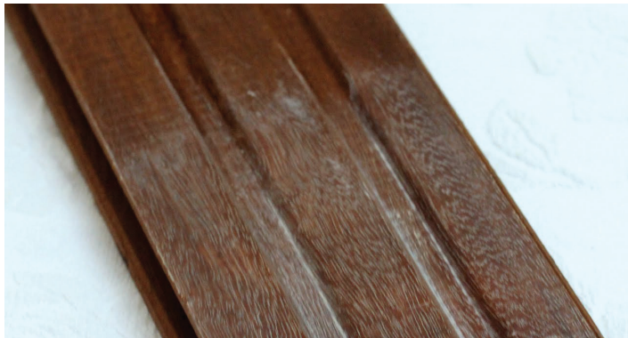
White Wax applied over bare timber
